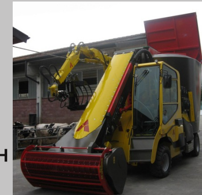
SUPER COMFORT CABIN WITH FRONT ENTRANCE THAT FACILITIES THE ENTRY AND GIVES THE POSSIBILITY TO WORK NEAR SILOS WALLS WITHOUT PROBLEM OF MOVEMENT AND EXIT
