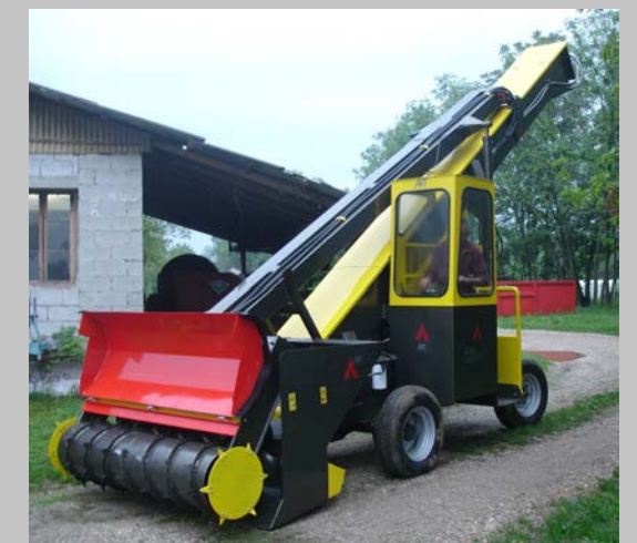
SELF-PROPELLED DE- ENSILER FOR CHARGING THE TRAILED MIXER WAGON
