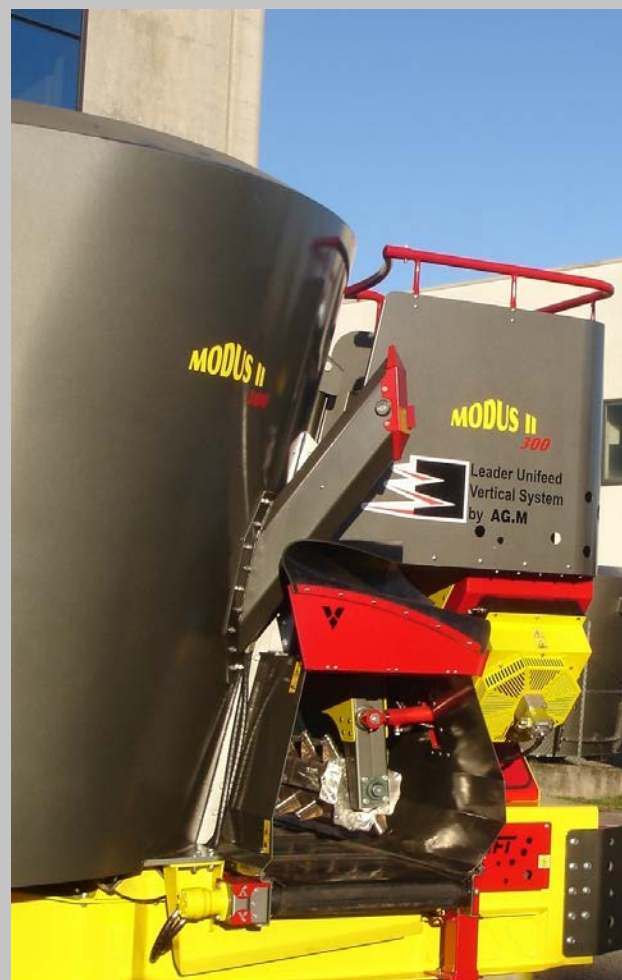
MAGNETIC DOSER ROLLER FOR AN HOMOGENEOUS DISCHARGE, PARTICULARLY INDICATED FOR DRY MIXING
