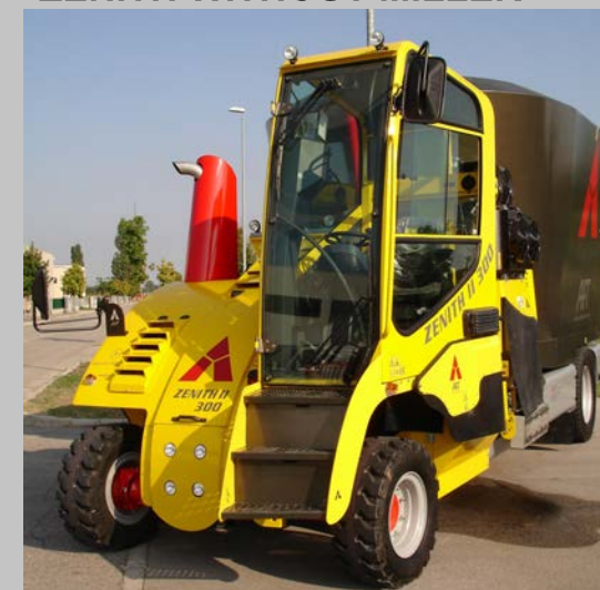
SUPER COMFORT CABIN WITH FRONT ENTRANCE THAT FACILITIES THE ENTRY AND GIVES THE POSSIBILITY TO WORK NEAR SILOS WALLS WITHOUT PROBLEM OF MOVEMENT AND EXIT
