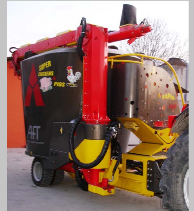
RAPID SUPER CHICKENS & PIGS EQUIPPED WITH RADIO CONTROL SYSTEM FOR THE AUGER UP TO 8 METERS OF HEIGHT. THE BEST FOR PIGS' OR/AND CHICKENS' BREEDINGS
