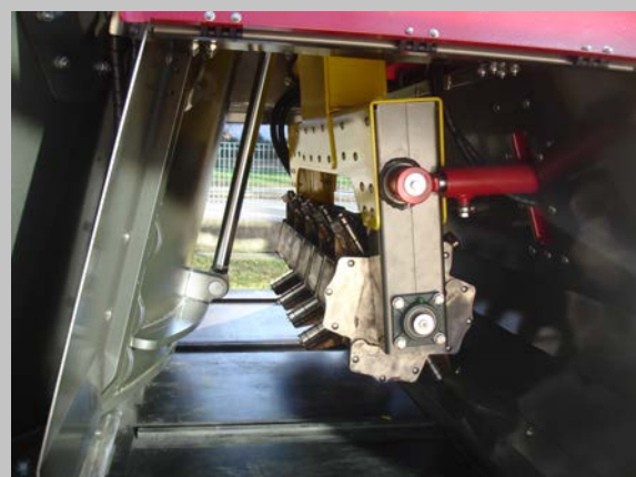
MAGNETIC DOSER ROLLER FOR AN HOMOGENEOUS DISCHARGE, PARTICULARLY INDICATED FOR DRY MIXING
