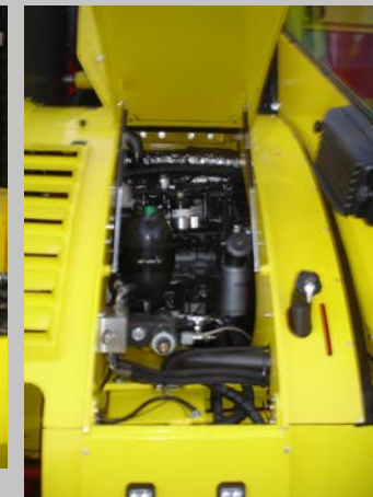
FULL ACCESSIBILITY TO THE ENGINE AND TO THE PUMPS
