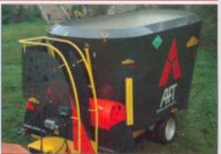
NUOVO CARRO VERTICALE TRINCIAMISCELATORE E DISTRIBUTORE, A 2 COCLEE DA 14 A 30 MC - ANCHE IN VERSIONE SEMOVENTE
